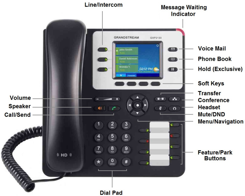
Figure 1 – Grandstream GXP2130 Telephone.
